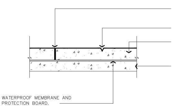
SEALTIGHT MEL-ROL SELF ADHERING WATERPROOFING MEMBRANE AND PROTECTION BOARD FROM W.R. MEADOWS, INC. IS ACCEPTABLE
